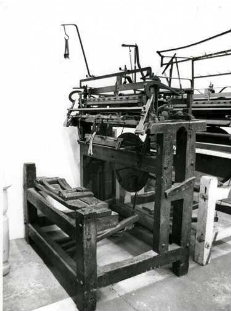
Associated image – picture of the framework knitting machine that will be on display, accession number NIM 1964-11.
